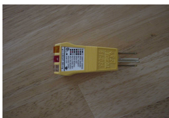
Fig. 5. Socket testers are typically used to verify the integrity of the power ground. Since these testers use the ac line as a reference, the socket tester results can be questionable and may even constitute a safety hazard.
