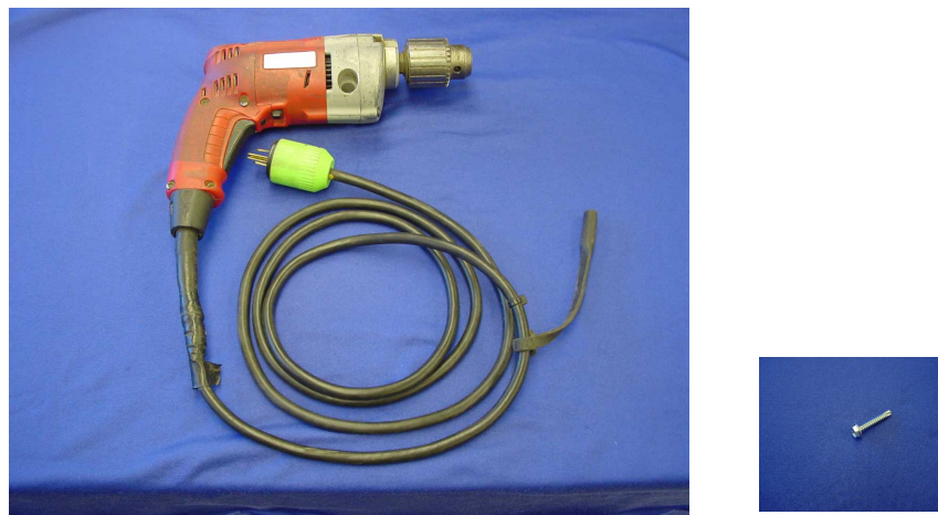
Fig. 3. Exemplar electric drill. The original molded three-wire, 120 Vac plug has been replaced by a different plug. On the right is a sheet metal screw similar to one found in the subject drill.
