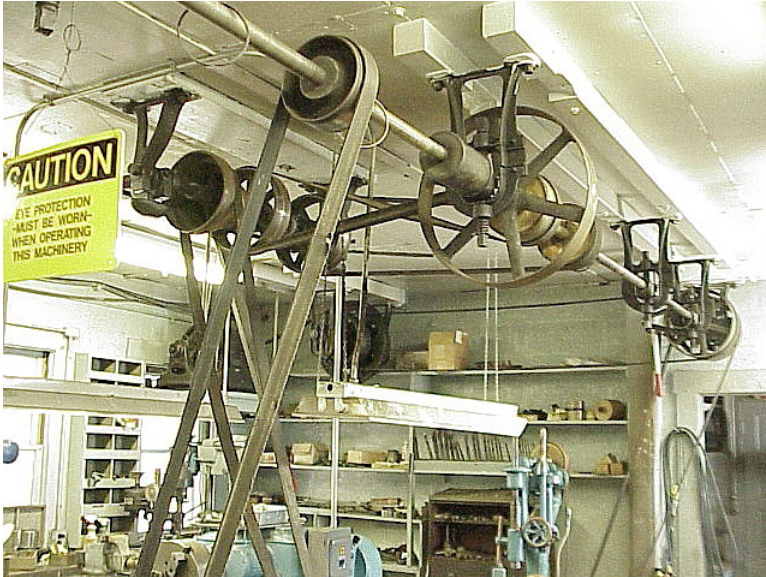
A Fitz Water Wheel and Belt Drive, Credit: Harry Matthews & http://www.old-engine.com
