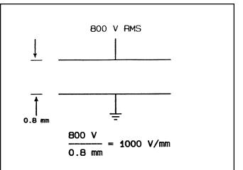
FIGURE 1A: Since 1000 V/mm is the same as the maximum withstand potential for air, this spacing will not break down.
