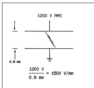
FIGURE 1B: Since 1500 V/mm exceeds the 1250 V/mm breakdown potential for air, this spacing breaks down.
