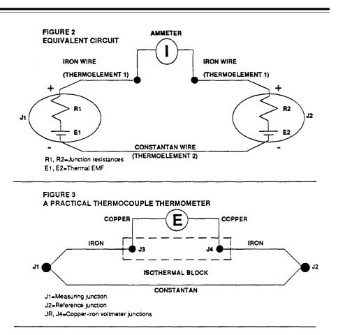
If the reference junction temperature is at 0 deg. C (in an ice bath), then, since the voltages in the tables are referenced to 0 deg. C, E2 = 0, and E = E 1. Now, we can eliminate the summing step, and just read the temperature directly from the tables.
