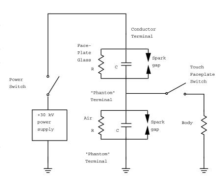
appear across the air than across the glass. If we assume the areas and distances of the two plates are equal for both the glass and the air, then about 87% of the voltage appears across the air, and 13% of the voltage appears across the glass.
